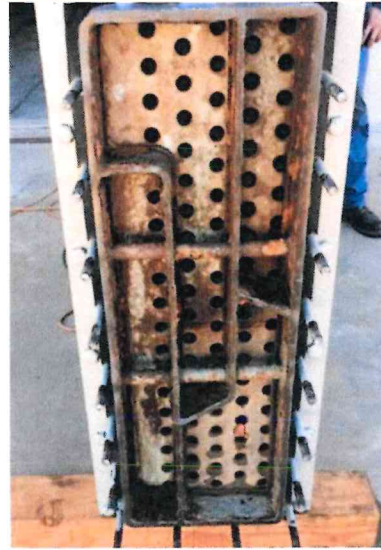
A Parker Dam heat exchanger before the HOD UV treatment implementation (left), and the same unit, exposed for the same time and similar conditions, after treatment with HOD UV (right).
